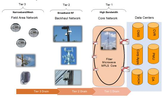
**Tier 1** represents the utility network core or backbone, a high-bandwidth network providing application aggregation and is woven throughout the utility territory. It consists predominantly of fiber optic and point-to-point microwave transport technology typically constructed in a ring topology for redundancy, with the majority of utilities using the 6 GHz spectrum band for the wireless segments. Fiber is the preferred transport medium; however, it is also the most
