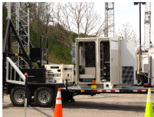
The SouthernLINC Wireless Storm Response Team uses a mobile cell tower to assist in storm response.
